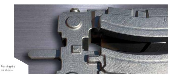
A large part covers the fabrication of pressing shop tools for autobody elements which are produced in the so-called natural mould method. 3D-cut patterns in polystyrene for single use are fabricated. During the casting procedure, they are transformed into high-efficiency cast tools. The material scope ranges from cast - and nodular iron to high-strength tool steels.
